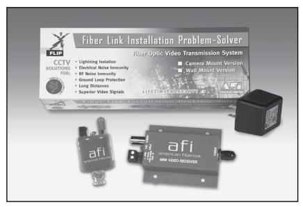
The American Fibertek VK-M1 and VK-M100 Video Kits transmit one channel of high-quality, FM video on one multimode optical fiber at 850 nm. Designed to be completely transparent to all camera and monitor manufacturers, the system requires no field adjustments at installation or additional maintenance thereafter. Diagnostic indicators provide a quick visual indication of system status
