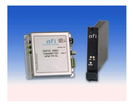
The American Fibertek M710SL Series transmits one channel of high-quality 10 bit digitized video on one singlemode optical fiber over a distance of up to 30 km. The rack card receivers are available in a single channel M710SL or a two channel M720SL configuration. The M720SL utilizes 2 fibers, one for each channel.
