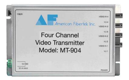
The American Fibertek 904 Series transmits four channels of high-quality 8 bit digitized video on one multimode optical fiber. Designed to be completely transparent to all camera and monitor manufacturers, this system requires no field adjustments at installation or additional maintenance thereafter. Diagnostic indicators provide a quick visual indication of system status. The "Afinety" intelligent remote monitoring system is available on this product, please consult factory.
