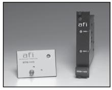
The American Fibertek M1410 Series is a low cost, low profile video and reverse data transceiver system. The video transmitter is specifically designed to plug into the back box of the Pelco Spectra camera dome. The system utilizes one multimode optical fiber to transmit video and return RS422 Protocol P or D for camera PTZ control. Designed to be completely transparent, this system requires no field adjustments at installation or additional maintenance thereafter.
