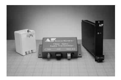
The American Fibertek 05B Series transmits single direction line level audio, 600 ohms balanced or unbalanced, on one multimode or singlemode fiber. The audio is transmitted over the link using FM modulation which results in an improved signal to noise ratio and a constant audio output level over the full optical loss budget. Diagnostic indicators provide a quick visual check of system status.
