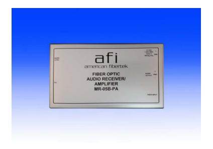
The American Fibertek 05B-PA receiver operates in conjunction with the American Fibertek MT-05B Series transmitters. The link accepts single direction line level audio, 600 ohms balanced or unbalanced, transmits the audio over one multimode or singlemode fiber and provides a 5W @ 70V output to power remote speaker systems.
