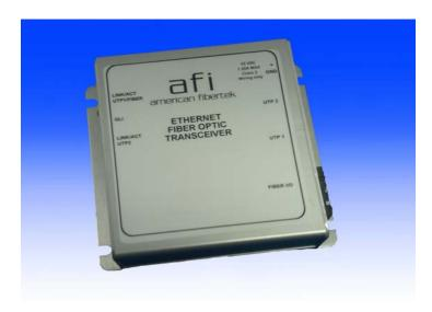
The American Fibertek 48-ZX Series transmits and receives (2) copper 10/100/1000Base-T Ethernet signals at the RJ45 ports and (1) optical 1000 Base-ZX over 1 or 2 singlemode fibers up to a distance of 70 km. The system is comprised of two units forming a communications link.
