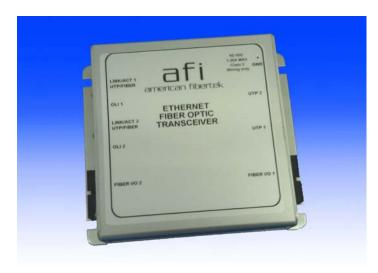
The American Fibertek 49-PoE-HP Series transmits and receives (2) copper 10/100 Base-T Ethernet signals at the RJ45 ports and (1) optical 100 Base-FX over 1 or 2 multimode fibers. The system is comprised of two units forming a point-to-point communications link.
