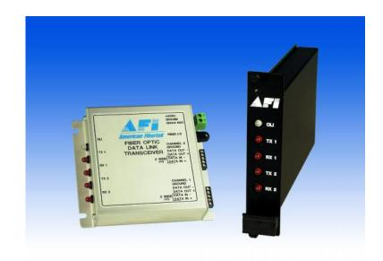
The American Fibertek 480SL Series transmits and receives one simultaneous channel of data over a single singlemode optical fiber. The system is comprised of two transceivers forming a point-to-point communications link. The system is designed to be completely transparent to data protocol and can be configured as RS-485 (2 wire or 4 wire), RS-422, RS-232 or Manchester Code. For ease of installation, diagnostic indicators provide a quick visual indication of system status.
