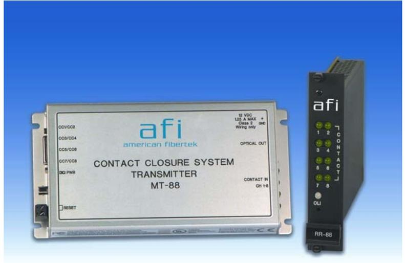
The American Fibertek 88 Series multiplexes 8 channels of "supervised input" dry contact closure on one multimode fiber. A set of 8 LEDs on the transmitter and the receiver units indicates the channel(s) status.
