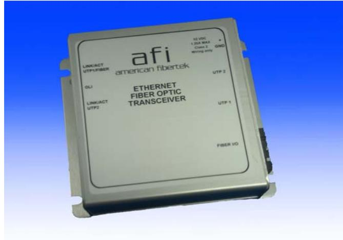
The American Fibertek 46-PoE-HP Series transmits and receives (2) copper 10/100 Base-T Ethernet signals at the RJ45 ports and (1) optical 100 Base-FX over 1 or 2 multimode fibers. The system is comprised of two units forming a point-to-point communications link.
