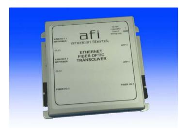
The American Fibertek 49-ZX Series transmits and receives (2) copper 10/100/1000Base-T Ethernet signals at the RJ45 ports and (2) optical 1000 Base-ZX over 1 or 2 singlemode fibers up to a distance of 70 km. The system is comprised of two units forming a communications link.
