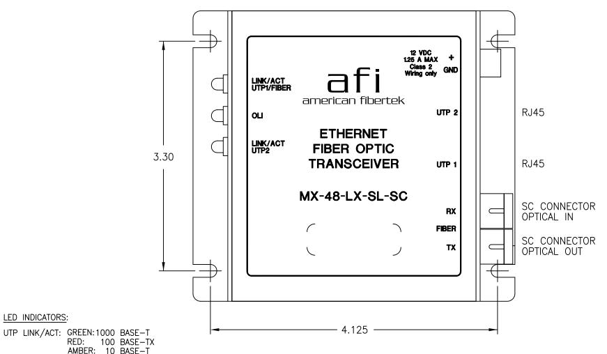
BLINK: UTP LINK IS ESTABLISHED AND ACTIVITY IS ON UTP PORT.
