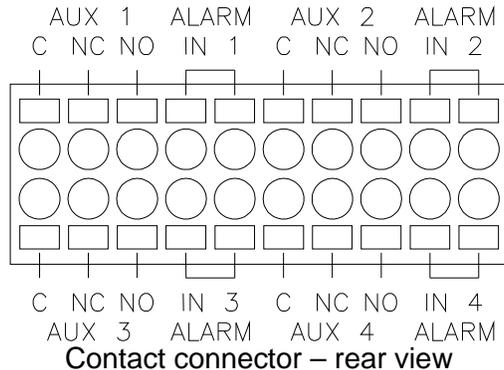
Each connector point on the block has a tab which is pressed in to insert / release the wire into the adjacent opening. To make a connection, strip ¼” from the end of a wire, then while pressing on the small orange tab adjacent insert the wire into the hole. When the tab is released the wire will be securely held in the hole. To remove the wire, press the tab again and pull the wire out.
