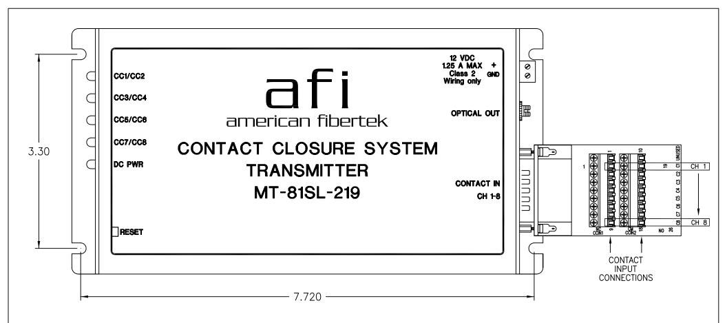
CC1 TO CC8 — CONTACT CLOSURE INPUT INDICATORS: GREEN INDICATES THAT THE CONTACT INPUT CONNECTION IS CLOSED.
