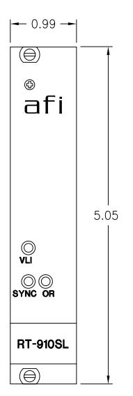
VLI — VIDEO LEVEL INDICATORS: SYNC — SYNC INDICATOR: INDICATORS ARE GREEN WHEN PROPER SIGNALS/LEVELS ARE PRESENT. THEY ARE RED WHEN SIGNALS ARE MISSING OR AT INCORRECT LEVELS.
