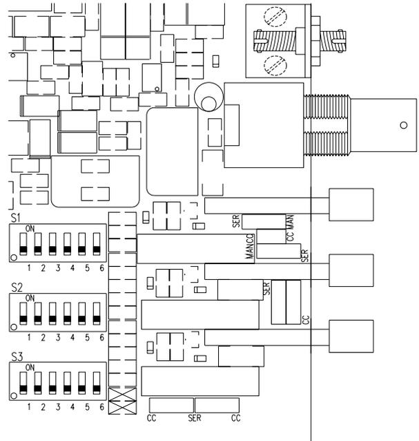
Please remember when using offset bias switches that they must be used in pairs. If switch # 1 is up then switch # 3 must also be up. The same situation applies for switch # 4 and switch # 6. Also, if using offset bias, it is important that the corresponding termination resistor switch be in the on (up) position. Using offset bias without a termination on the line will cause communications to fail. An explanation follows on general bias and termination guidelines.
