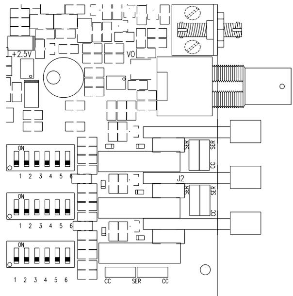
Please remember when using offset bias switches that they must be used in pairs. If switch # 1 is up then switch # 3 must also be up. The same situation applies for switch # 4 and switch # 6. Also, if using offset bias, it is important that the corresponding termination resistor switch be in the on (up) position. Using offset bias without a termination on the line will cause communications to fail. An explanation follows on general bias and termination guidelines.
