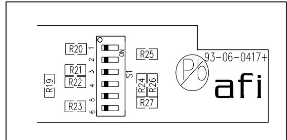
Please remember when using offset bias switches that they must be used in pairs. If switch # 1 is up then switch # 3 must also be up. The same situation applies for switch # 4 and switch # 6. Also, if using offset bias, it is important that the corresponding termination resistor switch be in the on (up) position. Using offset bias without a termination on the line will cause communications to fail. An explanation follows on general bias and termination guidelines.
