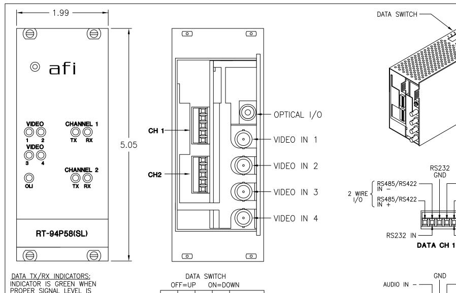
PROPER SIGNAL LEVEL IS PRESENT. OFF WHEN SIGNAL IS MISSING OR AT AN INCORRECT LEVEL.
