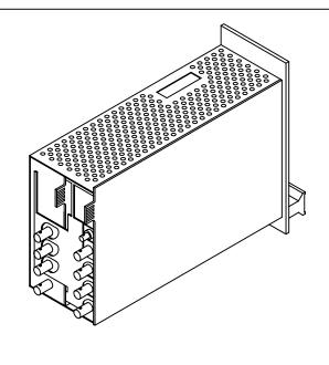
VIDEO — VIDEO LEVEL INDICATORS: INDICATORS ARE GREEN WHEN PROPER SIGNALS/LEVELS ARE PRESENT. THEY ARE RED WHEN SIGNALS ARE MISSING OR AT INCORRECT LEVELS.
