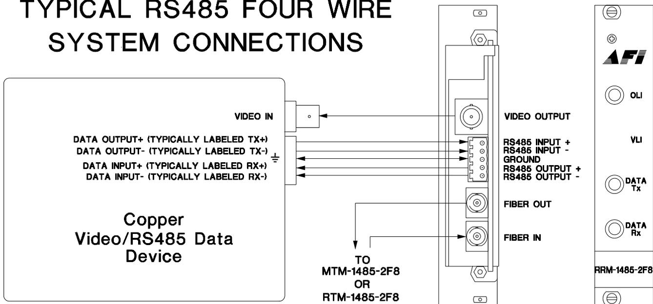
Also, please note that in four wire installations Data In on the RRM-1485-2F8 becomes Data Out on the MTM-1485-2F8 or RTM-1485-2F8 after going across the fiber. The reverse flow follows the same orientation.
