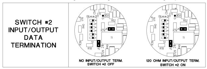
To open the MTM-61, remove the screw on the bottom of the module. Also remove two screws holding the end panel to the chassis on the side with the video and data connections. Slide PCB assembly out of chassis to access the switch and jumper locations.
