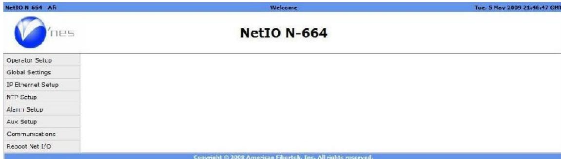
The N-664 web interface screens use a common design in which the screen is divided into three sections. Across the top of the screen is a title bar which contains the user-settable device name and device location strings, and the current time and date setting.
