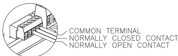
The contact blocks have three terminals which are used for the aux contact out function. The contact outputs are form C contact closures.
